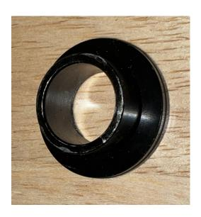
The stepped spacer fits through the large washer, which then sits FLUSH against the wheel bearing. Don't worry about the alignment of the internal tube, and you may have to straighten it. The bearings may need to seat after the first time you install the wheel, but this will happen as you tighten the axle. Here are some detailed pictures to help:
