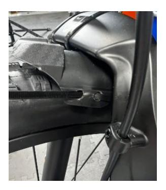
Front fender positioning under the fork.
