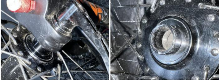
Now, insert the wheel between forks and align the holes on the wheel/spacers with the holes in the forks. CAREFULLY align the brake rotor into the front brake caliper. from right (non-disk) side. It should fit easily, but if there is slight rubbing when spinning the front wheel, we will adjust the brake caliper (see below, only if necessary). Rotate using handle (handle can be pulled out, counter-rotated and re-engaged to tighten) Rotate crank handle clockwise by hand until tight.
