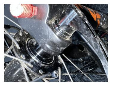
Now, insert the wheel between forks and align the holes on the wheel/spacers with the holes in the forks. CAREFULLY align the brake rotor into the front brake caliper. from right (non-disk) side. It should fit easily, but if there is slight rubbing when spinning the front wheel, we will adjust the brake caliper (only if necessary). Rotate using handle (handle can be pulled out, counter-rotated and re-engaged to tighten) Rotate crank handle clockwise by hand until tight.
