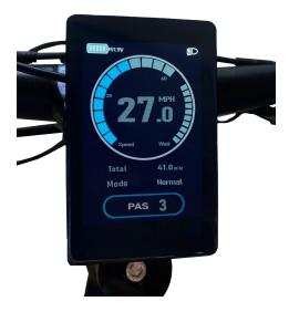
The LCD control panel display provides real-time information on PAS (Pedal Assist) level, power consumption, remaining battery level, battery voltage, and light indicator.
