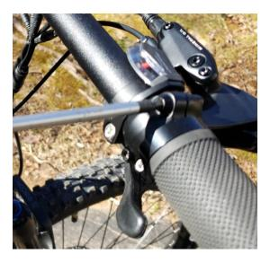
Adjust the brake lever position. Too close and it will hit the bar before fully engaging brakes, too far backwards or forwards and it will be difficult to reach:
