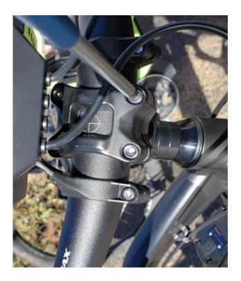
Adjust your shifter (right) and brake lever positions up and down (left and right bar):
