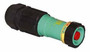
The new Rotalock system provides an excellent solution to this problem. Uncoupling is achieved by simply rotating a coupling ring. When rotated the coupling ring moves in a lateral plane to disengage the locking pin. In this way no separate tools are required for uncoupling.
