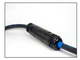
This device allows a simple and cost effective method, via which two cable ends fitted with standard crimp lug, can be connected together. A bus bar is retained within a threaded section and via two bolts the lugs are connected to the bus bar. The outer housings and cable glands are then screwed onto the retainer, to provide a watertight enclosure around the connection. The housings are manufactured from high impact high dielectric insulation material for user safety and long life.
