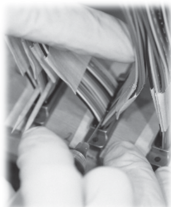
Potting a Micro-D with Epoxy-Filled Syringe
