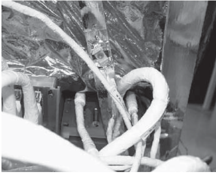
Detail of the Atmospheric Infrared Sounder Instrument (AIRS) with Glenair Micro-D Cables and Connectors
