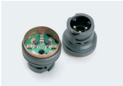
Pressure transmitter sensor-connector with PCB terminals. (Other termination methods are possible). Connector is fixed either by flared joint or overmold.
