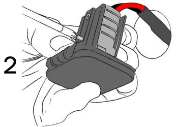
Feed the Anderson lead out through the panel hole and install the plug into the mount.
