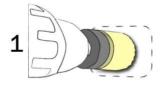
Locate the ideal position for the mount and drill the 38mm central hole.
