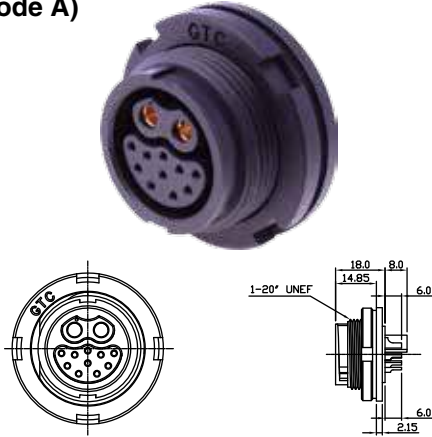
Hybrid C4 25A+5A 2P+10P Panel Female Solder Lock (Code A)
