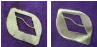
Deburring with wide abrasive belt and double sided edge rounding with cross belts
