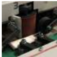
Option: counter rotating lamella brushes available for edge rounding after side grinding
