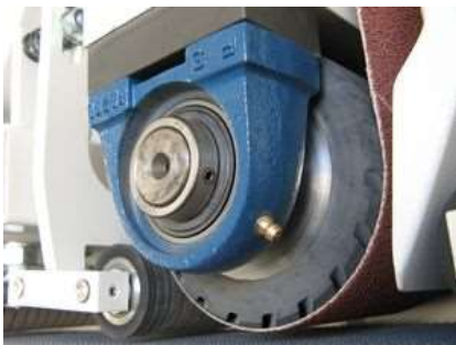
Abrasive belt head with contact roller
