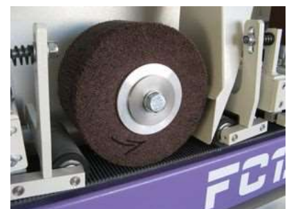
Abrasive brush for a smoother finish after belt grinding
