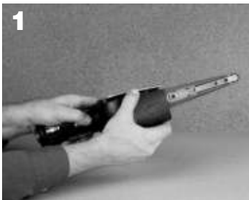
1 With your thumb, pull and slide guard open in a clockwise direction.
