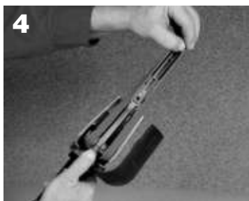
4 Slip belt over contact wheel. Release idler arm lever. Operate on the contact wheel or on the return side of the belt.
