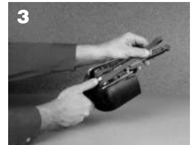
3 Depress idler arm lever and pull belt toward the contact wheel.
