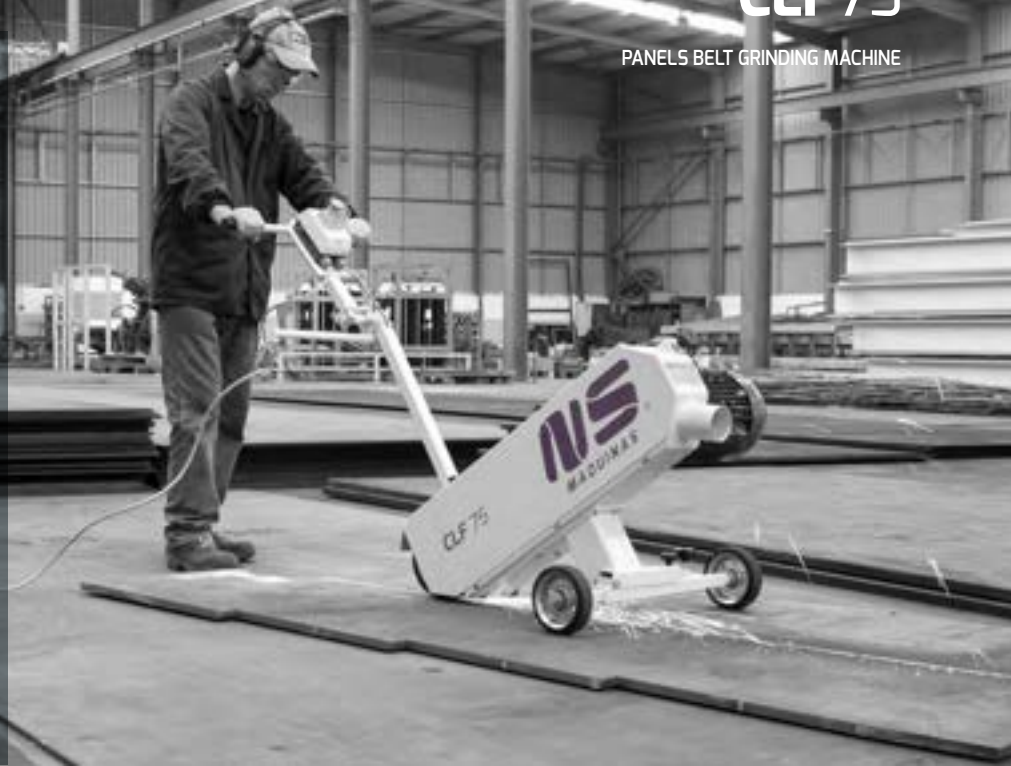
Weld seam and heavy sheets grinding
