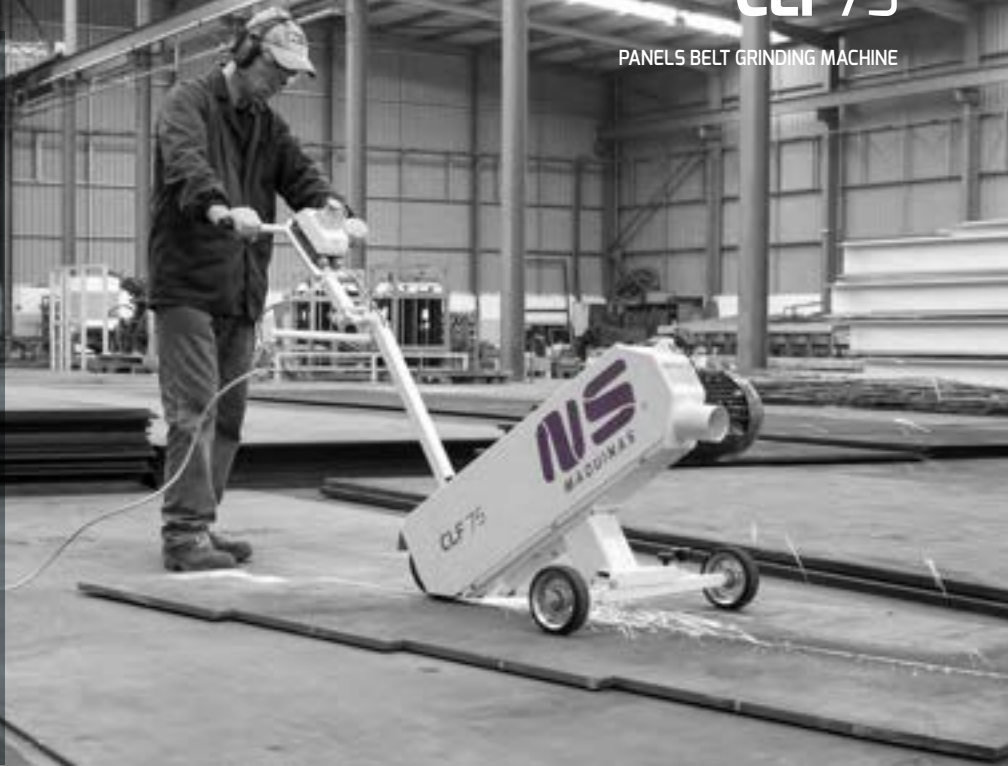
Weld seam and heavy sheets grinding
