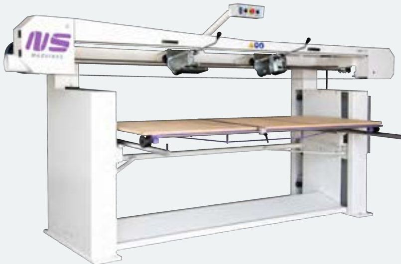
Boxes and welded structures belt finishing
