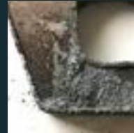
Smooth edges with a radius from two counter rotating abrasive cross belts
