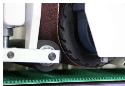
Pressure rollers before and after each abrasive station
