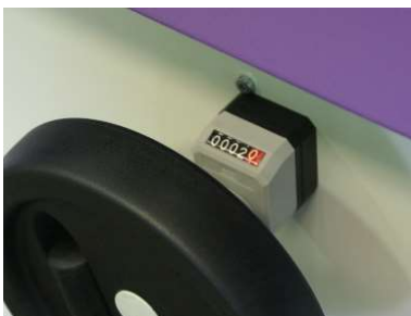
Pressure and thickness adjustment with 1/10mm precision
