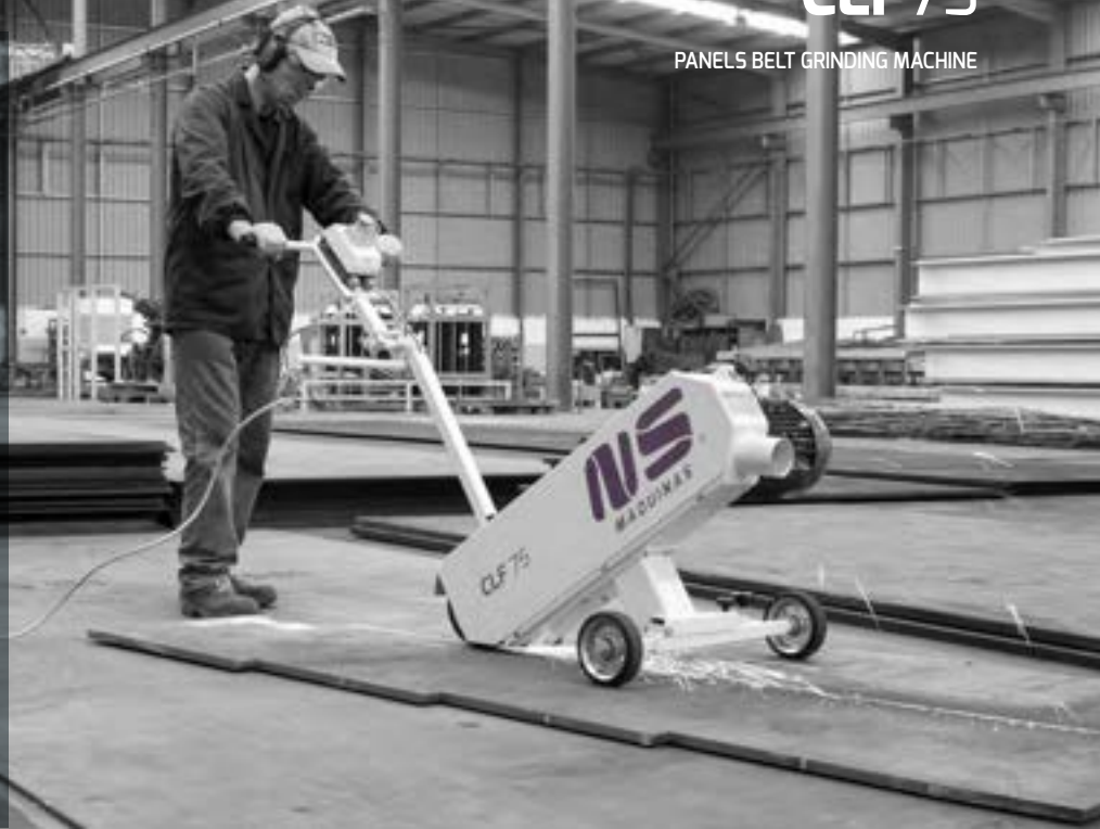
Weld seam and heavy sheets grinding
