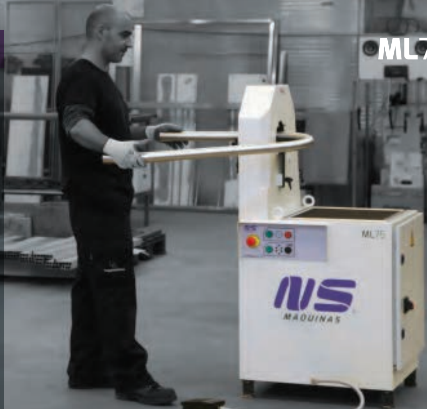
Finishing tight curved tubes with diameters up to Ø76mm
