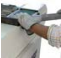
Top abrasive belt section for tube end deburring
