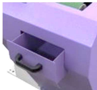
Dust collecting drawer at conveyor belt exit
