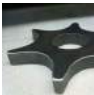
Rounding edges of thick plate steel parts
