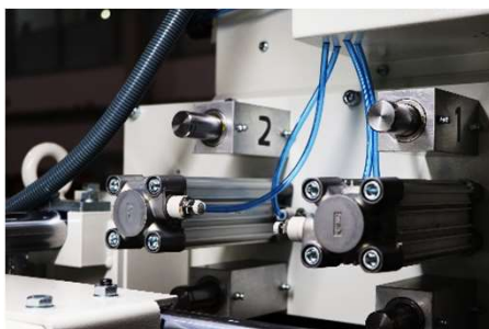
Pneumatic tensioning for both grinding belts
