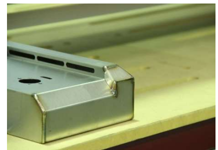
Surface finishing and weld grinding of flat surfaces and corners
