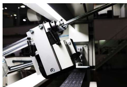
Contact roller with width adaptability assembled on counterweight system
