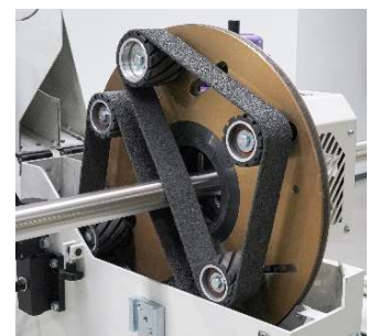
Planetary wheel with 2 abrasive belts
