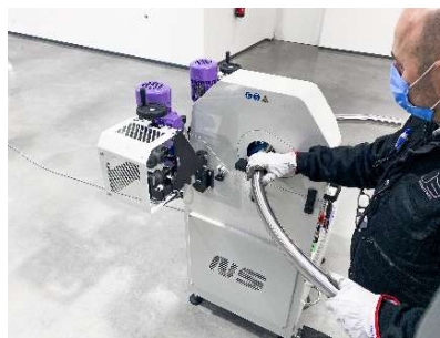
Easily removable feeding units for bent tube finishing
