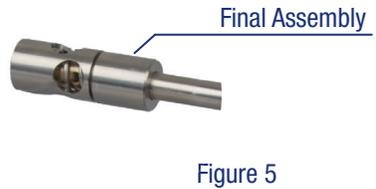
6. Secure the Collet using the 3/32" hex key through the hole in the brass Collet and rotate it clockwise to tighten the Collet. The Collet should be firmly fitted but not overtightened. Only apply light pressure when tightening.
