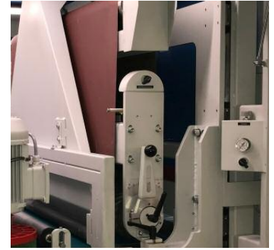
Abrasive belt unit with floating head system
