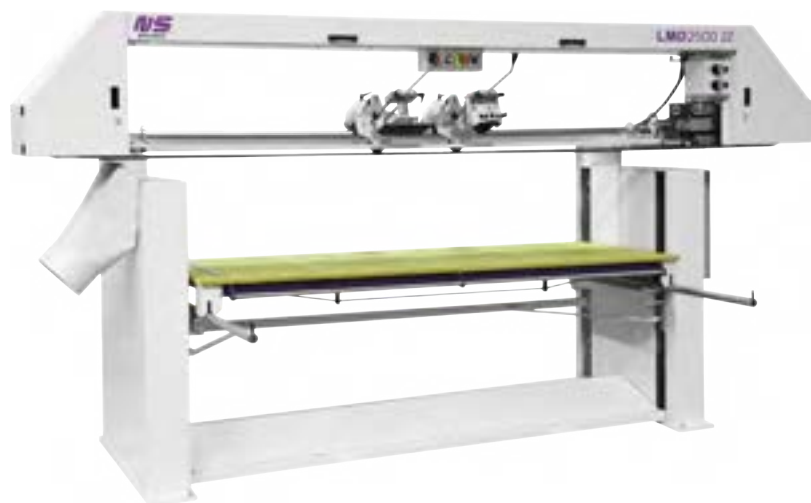
Pneumatic abrasive belt tensioning
