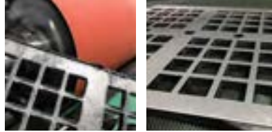
Large deburring drum as alternative to remove heavy burrs and slag
