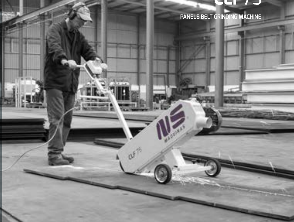
Weld seam and heavy sheets grinding
