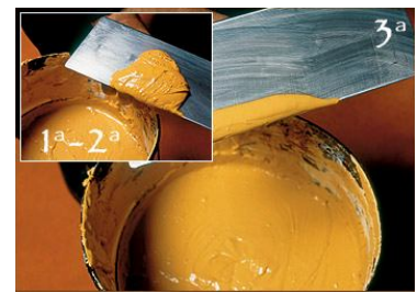
Step 6 - Here is a picture of the two different consistencies. Use our special spatulas, especially for the third coat.
