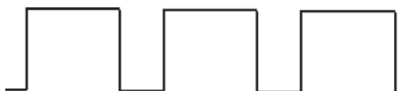
Forward power sensor signal waveforms
