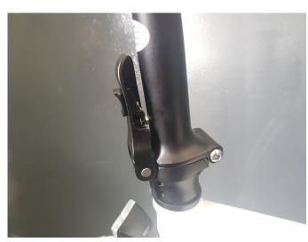
Fold the main clamp upwards until it 'clicks' into position.
