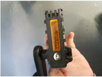
Rotate the pedal upwards to fold the pedal. To unfold the pedal just rotate the pedal back to its normal position and you should hear a click.
