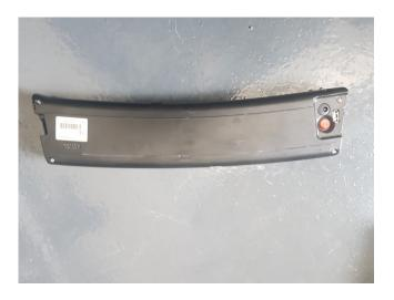
Insert the key in the hole and turn. The battery will unlock from the frame and allow the battery to be removed from the frame of the bike. Once the battery has been removed you can store it or charge it as you so desire. To reinstalled the battery. Just reinsert it into the frame and lock the battery with the key.
