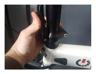
Locate the folding mechanism for the handlebars this can be seen in the top left picture. Rotate the plastic safety latch around anti clockwise to release the main latch as shown in the top right picture.
