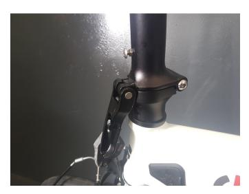
Locate the handlebar folding joint, this can be seen in the top left picture. Rotate this upwards to close the folding joint. Please note also that the allen bolt shown in the top left picture will adjust the steering alignment tension and may require a small amount of adjustment after the handlebars have been installed.
