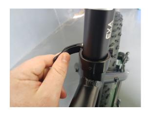
adjust the tension of the clamp. To do this while the clamp is open rotate the clamp clockwise to tighten. Attempt to close clamp again at the desired tightness. If you are unable to close the clamp is may be too tight and require loosening. Check the maintenance document for more details.
