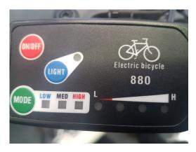
To turn the LCD on, hold down the power button for half a second, the light will flash and turn on. Battery meter is displayed in the bottom right and the pedal assistance level shown on the bottom right.
