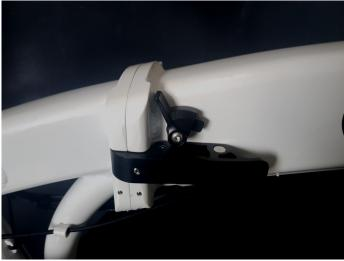
Locate the folding latch and lift the black safety latch upwards. Open the chrome latch outwards to unlock the folding mechanism.
