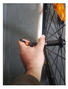
Close the axle clamp to lock the wheel on the bike. If this is quite easy to do you may need to tighten the nut a little more until it is firm clamp.
