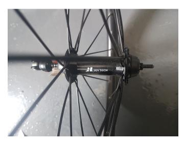
Insert the axle through the front wheels hub and loosely screw on the nut. Ensure that you insert the spring on before the nut. You can now place the front wheel in the front forks of the bike. Insert the wheel as shown below. Tighten the quick release mechanism by tightening the nut on the axle.
