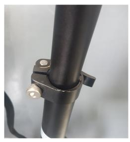
Insert the handlebar to the desired height ensure that the engraved maximum handlebar height is not visible. (insert them below the clamp). The maximum handlebar height markers are shown in the top right picture. Close the clamp as shown in the bottom two pictures. If this is too hard or two easy to close you should adjust the tension of the clamp by tightening the thumb screw while the clamp is open. This will ensure that the clamp is firmly closed and no nuisance movement will occur.
