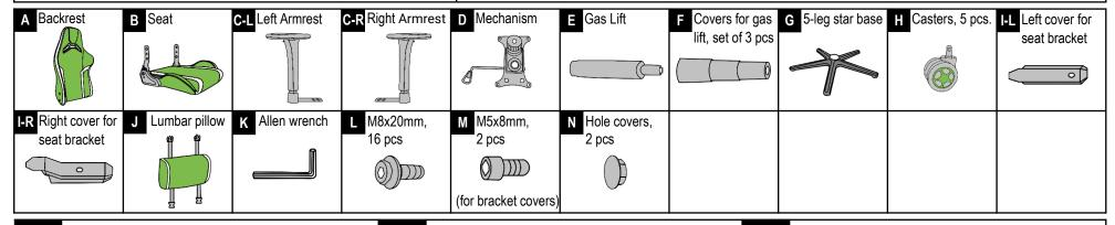
STEP 1 Insert the casters H into the legs of the base G using pressure, then place the gas lift E in the middle of the base and cover it with F.
