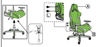
STEP 5 Attach the covers (I-L) and (I-R) to the brackets on their respective sides of the seat (B) using screws (M) and cover the holes with (N) as shown.
