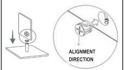
3. The panels might have a very small gap which is normal; turn the cam lock clockwise to lock the parts together and the gap will also close.
