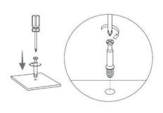
2. In the other panel, insert the cam lock and align it so it can properly receive the bolt, then join both panels (the cam locks might come pre-installed in this unit).
