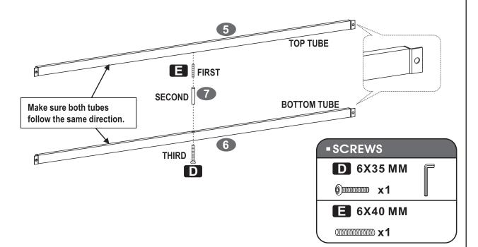
Using screws (A) and O'rings (G), assemble the structures (5) and (6) to the structures in "L" (8) and (9) as shown. You can now proceed to tighten the screws (D) and (E) from the previous step.
