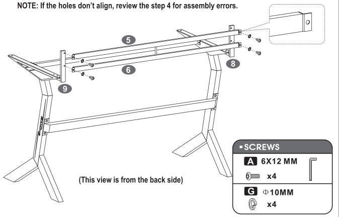
Pay attention to the correct screws that will need to be used. To avoid misalignments, first place all the screws loose.
