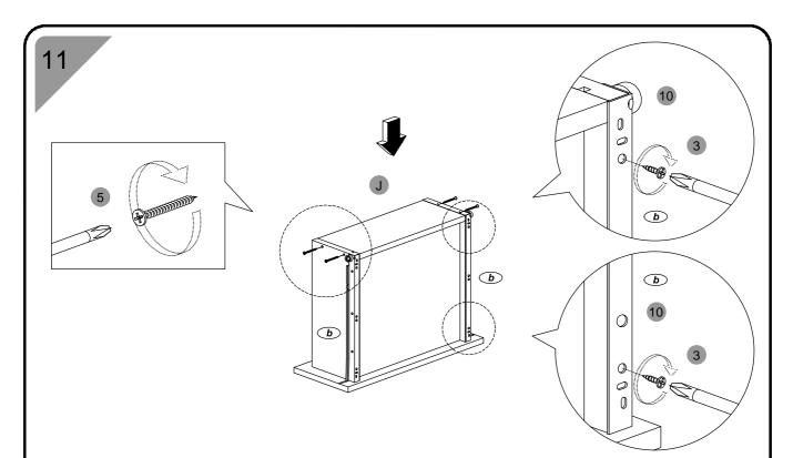
• Install panel (J) with screw (5) on both sides. Then attach Metal Sliders (10b) with screw (3) to Left & Right side as shown above.
