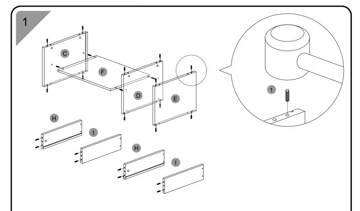
• Install 24pcs of Wooden Pins (1) into all panels as shown.
