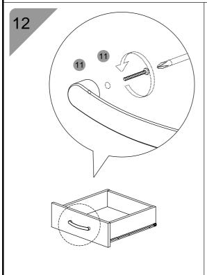
Attach Handle (11) with screw for handle as shown above.
