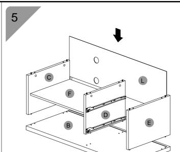
Place panel (C),(D),(E) & (F) on top of bottom panel (B). Then, Insert back panel (L) between panels (C) & (E) as shown.
