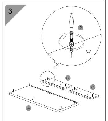
Attach Cam Lock (2) to panel (A) & (G) as shown above. **RTA-8896** P.4
