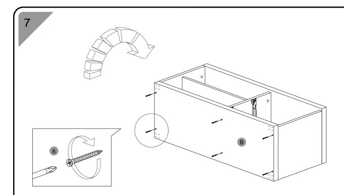
• Place the unit on its side and secure bottom panel (B) with screws (6).
