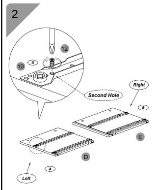
Attach Drawer Metal Sliders (10a) to panel (D) & (E) using screw (12).
