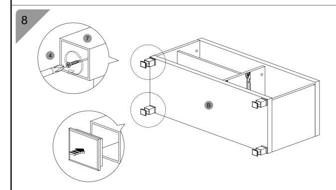
• Install Plastic Feet (7) using screw (4) to bottom panel (B). Make sure once these are attached to cap them off with the plastic caps as shown above.
