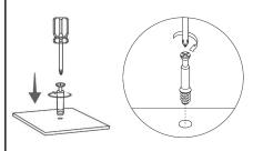
2. In the other panel, insert the cam lock and align it so it can properly receive the bolt, then join both panels (the cam locks might come pre-installed in this unit ).
