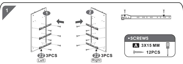
• Grab all the flat shaped Drawer Sliders (22) and set aside the "L" shaped ones. With the Left & Middle Panels (1&2) oriented as illustrated, assemble the flat sliders (22) to the holes on their inside faces. The wheels will be located at the front and facing down.
