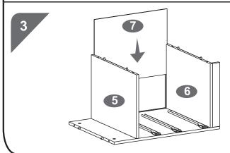
Slide in the Back Panel (7) thru the channels in between the Horizontal Panel (5) and Bottom Panel (6) as shown. Make sure the panel fits inside all the channels.
