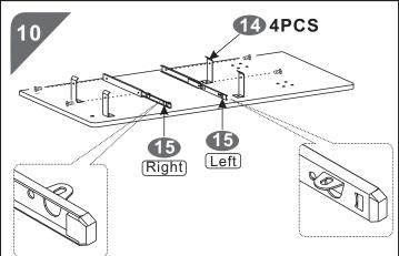
Use Screws (G) to fix the Keyboard Slider (15) to the Slider Bases (14) as illustrated. Please note the position of the tabs on the sliders.
