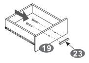
Assemble the Handle (23) to the Drawer Front Panel (19) using Screws (K) as shown.
