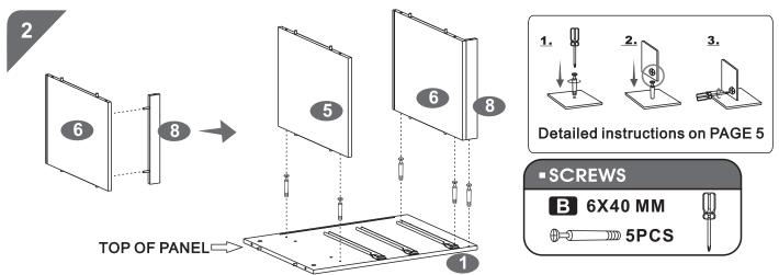
•Join the Front Base Panel (8) to the Bottom Panel (6) by inserting the wood pins of (8) into the holes of (6) as shown.
