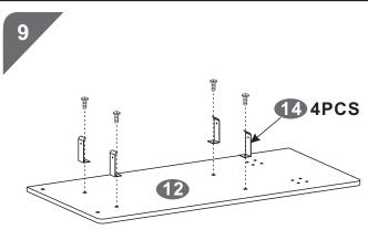
■Use Screws (F) to affix the Slider Bases (14) to the Main Panel (12).
