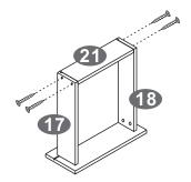
Assemble the Drawer Back Panel (21) between the Drawer Left & Right Panels (17&18) using Screws (J) as shown.
