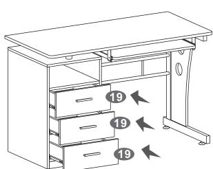
Carefully insert all the drawers starting from the bottom. Make sure the wheels from the drawers engage and roll in the middle of the sliders.
