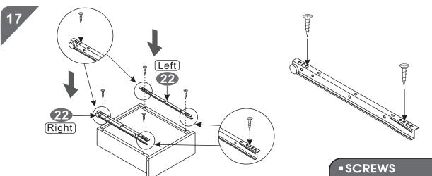
■ Place the drawer upside-down. Grab the "L" shaped sliders (22) and assemble them to the drawer using Screws (A), with wheels facing towards the back of the drawer. Make sure the sliders are touching the side panels, and that they are not "up in the air".
