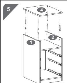
Screw the Bolts (B) to the corresponding holes on the inside face of Top Panel (4), then assemble it to the cabinet by turning the corresponding cam locks.
