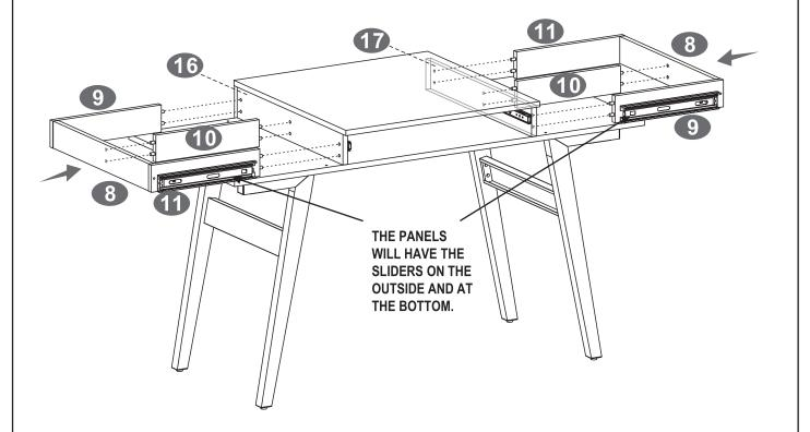
Using screws (G), and from beneath the unit, assemble the panels (8), (9), (10) and (11) to the bottom panel (7) as shown.
