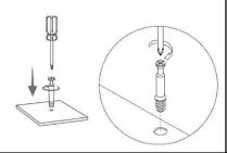
2. In the other panel, insert the cam lock and align it so it can properly receive the bolt, then join both panels.
