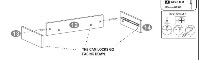
Using bolts (A), assemble the panels (12), (13) and (14) to the panel (15) as shown and as explained in page 4. **REPEAT THE STEPS 14 THRU 16 FOR THE SECOND DRAWER.**
