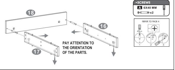
Using bolts (A), assemble the panels (16), (17) y (18) to the top panel (19) as shown and as explained in page 4.
