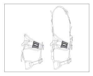
• On the multi-standard NAVAHO and AVAO harnesses, check the fall arrest indicator. The indicator shows red if the dorsal attachment point sustains a shock load greater than 400 daN.
