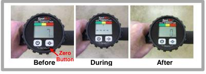
With the meter powered on, hold the meter above the ground with the shaft facing down. Press the **ZERO** button and continue holding the meter steady and above the ground until the zero function completes and the LCD displays a "0" value.
