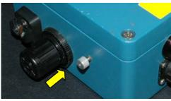
b) Press the finger switch once to engage the handpiece piston.
