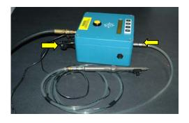
9) Turn on the power to the control box using the green on/off button.
