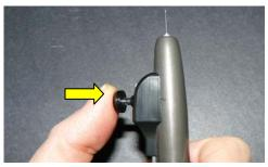
11) Increase the air pressure to a normal operating level between 40 psi and 80 psi. (Unlock the air pressure regulator knob by pulling it out; set the air pressure to the desired level; relock the air pressure regulator knob by pushing it in.)
