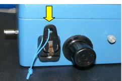
8) Attach the completely assembled handpiece (see section 4 for instructions) to the control box by connecting the clear air hose to the handpiece air quick connect on the front of the control box and the black handpiece cable to the handpiece connector on the back of the control box.
