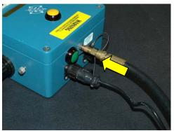
7) Insert a charged token into the token port on the side of the control box.
