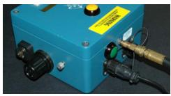
2. Disconnect the handpiece air hose from the control box.
