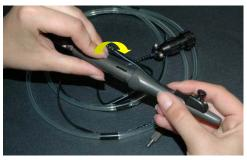
c. Once the threads have separated, pull the cylinder body and the syringe housing apart and remove the injection syringe with needle and piston. Occasionally, the injection syringe will stick in the syringe housing. It can be dislodged by pushing down at the base of the needle against a flat surface such as the edge of a table or flat edge of a screw driver.
