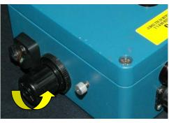
c) Lock the air pressure regulator knob by pushing it in.
