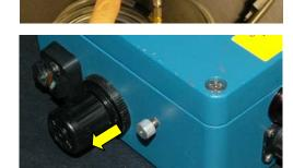
iii) Turn the air pressure regulator knob clockwise to increase the pressure until 20 psi is reached.
