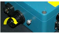
iv) Lock the air pressure regulator knob by pushing it in.
