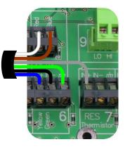
In DeltaLINK<sup>4</sup> configure channel 6 as type **ML3** and channel 7 as a type **ML3 Temperature** sensor.
