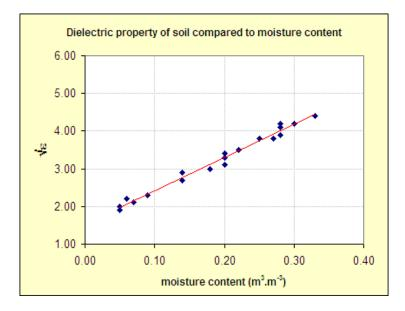
The goal of calibration is to generate two coefficients ( $a_0$ ,  $a_1$ ) which can be used in a linear equation to convert probe readings into soil moisture:
