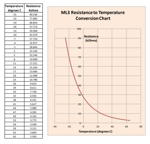
Note: This table has been optimised for use as a look-up table. To minimise linear interpolation errors the data points fall either side of the manufacturers' specified sensor response curve. This helps optimise the overall accuracy of readings.
