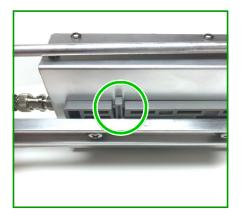
To detach the receiver from the antenna, push the release latch on the antenna mount and slide the receiver from the antenna. When re-attaching, slide the receiver forward until a small click is felt.
