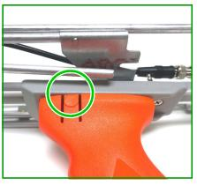
The handle slides into the bracket beneath the antenna and will lock into place with a small click. To remove handle, depress the release button and slide the grip free.
