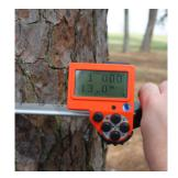
The MD II computer is rugged and field adapted. Communication and data transfer to external devices is convenient and made with USB cable and Bluetooth<sup>®</sup>.
