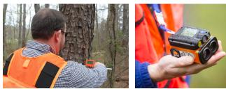
The MD II caliper is adapted for efficient field measurement work. Register diameters, input tree species and send tree heights with IR from the Vertex IV or VL5 instruments. Collect all data in the non-volatile internal memory or transfer online with Bluetooth® to handheld computer, tablet or mobile phone.
