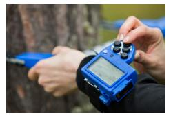
The DP II computer terminal placed on the wrist and with the SmartScale used to measure standing tree diameters. This work mode is possible by using the Radio Enter button (factory assembled) on the SmartScale to send data to the computer terminal for storing and processing.
