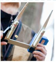
The image shows Gator Eyes laser pointers installed on the Digitech Professional caliper. When Gator Eyes are installed, the total weight of your caliper will increase with approx. 190g./7,6oz.
