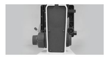
2. Unscrew four Allen hex socket cap screws holding back cover plate.
