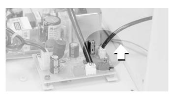
3. Disconnect the LED connection cables from the power supply printed circuit board.
