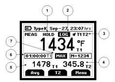
The dot matrix display features a large primary display, smaller secondary displays for channel info or min/max/ave, and helpful annuciators for added measurement data
