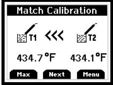
Use the ▲ or ▼ keys to adjust the value to match T1 readings and T2 readings.
