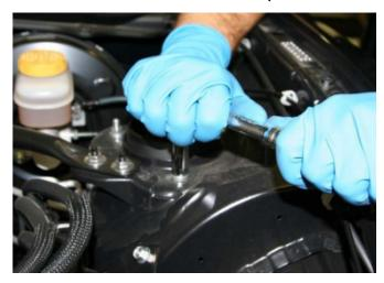
6. Once all three 12mm top nuts are removed, ensure the abs and brake line are out of the way and remove the strut from the car.
