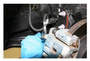
3. Remove 17mm nut that attaches swaybar endlink to strut using a 17mm open end wrench and a 6mm allen key.
