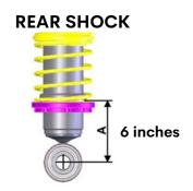
50mm threads bottom spring perch to end of threads
