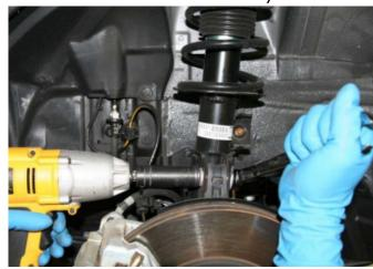
5. While having the strut supported or held in place, carefully remove three upper 12mm nuts that fasten strut top mounts to chassis.
