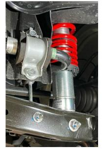
8. Install and torque wheels. Roll the car on level ground and check ride height. Adjust if needed
