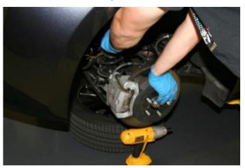
NOTE: If there is still too much tension to remove the shock, remove the 17mm nut/bolt that connects the swing arm to rear hub
