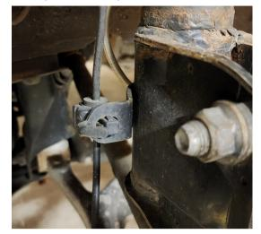
2. Remove 12mm bolt that attaches the brake line
