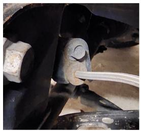
4. Remove the two 19mm nuts/bolts that attaches the front strut to the hub
