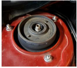
6. Once all three 12mm top nuts are removed, ensure the abs and brake line are out of the way and remove the strut from the car.
