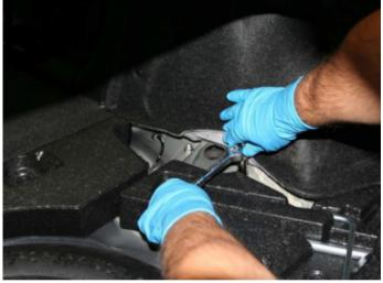
3. Remove 17mm bolt/nut that attaches the shock to swingarm (1) and 14mm bolt/nut that attaches swaybar endlink to swingarm (2)
