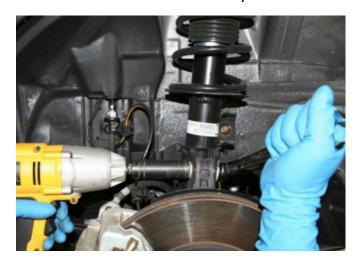
5. While having the strut supported or held in place, carefully remove three upper 12mm nuts that fasten strut top mounts to chassis.
