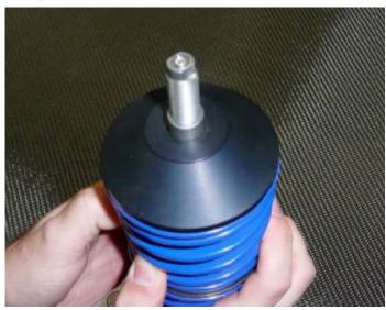
2. Install OEM conical washer on top of upper spring perch.
