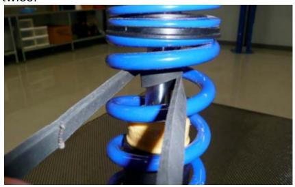
5. Twist and hold the strap tightly. Torque top nut to 26ft-lbs
