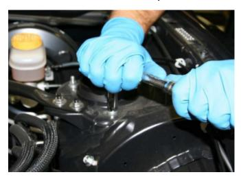
6. Once all three 12mm top nuts are removed, ensure the abs and brake line are out of the way. Carefully remove OEM strut from the vehicle.
