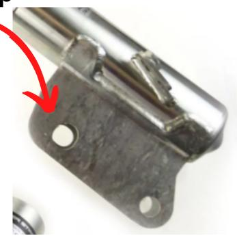
DO NOT use an aftermarket camber bolt on the UPPER slotted upper strut hole.IF additional camber is needed, an OEM crash bolt is recommend. An aftermarket camber bolt may be used for the LOWER bolt.
