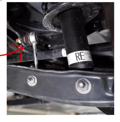
**3.** Remove (4) 12mm nuts that secure the sway bar mount to the chassis and carefully pull out the OEM sway bar along with the mounting brackets.
