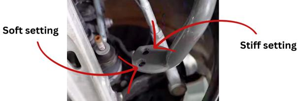
**10.** Fully tighten all loose bolts. (4) 12mm bolts securing the sway bar bracket to the chassis and (2) 17mm end link nuts and re install both front trays.
