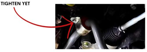
9. Once you have determined the desired stiffness for your vehicle, carefully guide the sway bar end link through the desired hole and reinstall the 17mm nut on the end link. Repeat on
