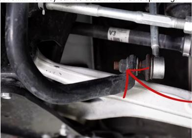
Remove 17mm nut on each side (step 3)
