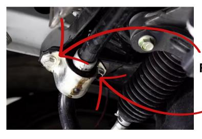
Remove 12mm bolts (2) on each side
